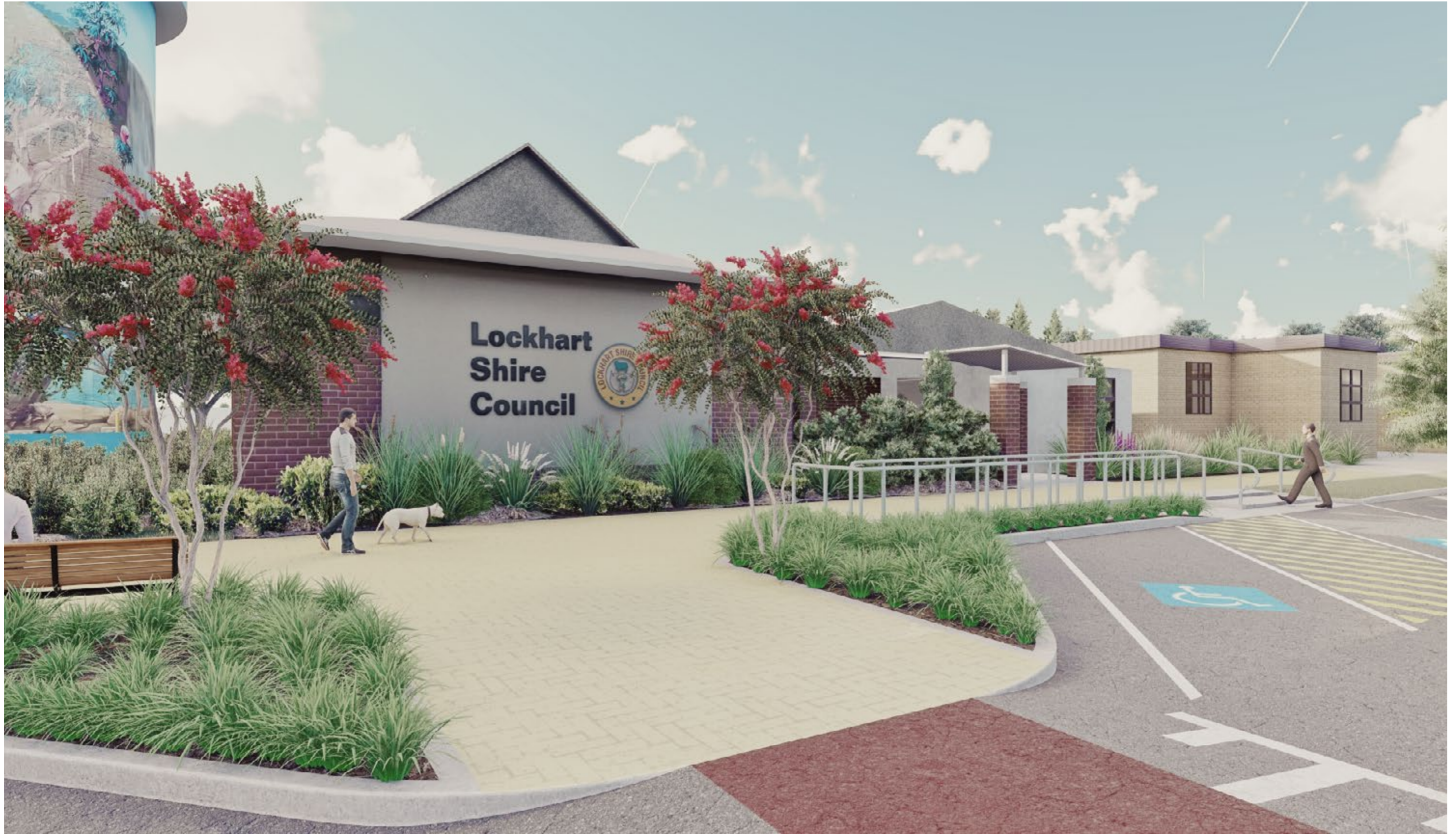
d Extended kerbs and paving, raised pedestrian access-way, furniture and steps provides a way to integrate the existing disabled ramp into the streetscape.
