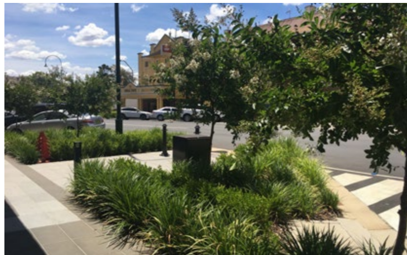
Example of a kerb out-stand with street furniture and planted with small street trees and evergreen tufting plants.
