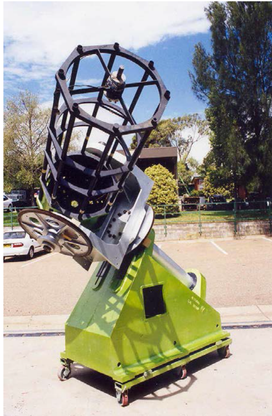
The 24 inch research telescope for TRRO. Principal usage will be double star astrometry.
