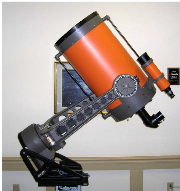
The C14 telescope. A 14 inch aperture Schmidt Cassegrain telescope with very good optics suitable for double star astrometry, quasar photometry and general viewing.
