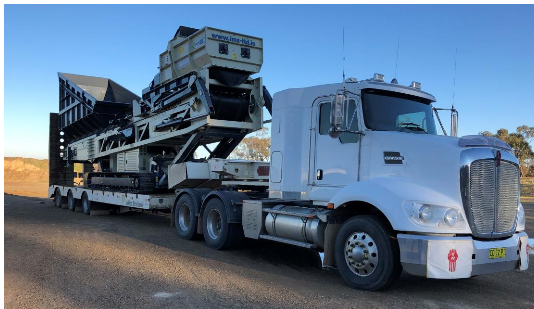
A grant from the NSW Environment Protection Authority enables Council to purchase a Pugmill which will be used to blend crushed glass to be used in Council's road base material.
