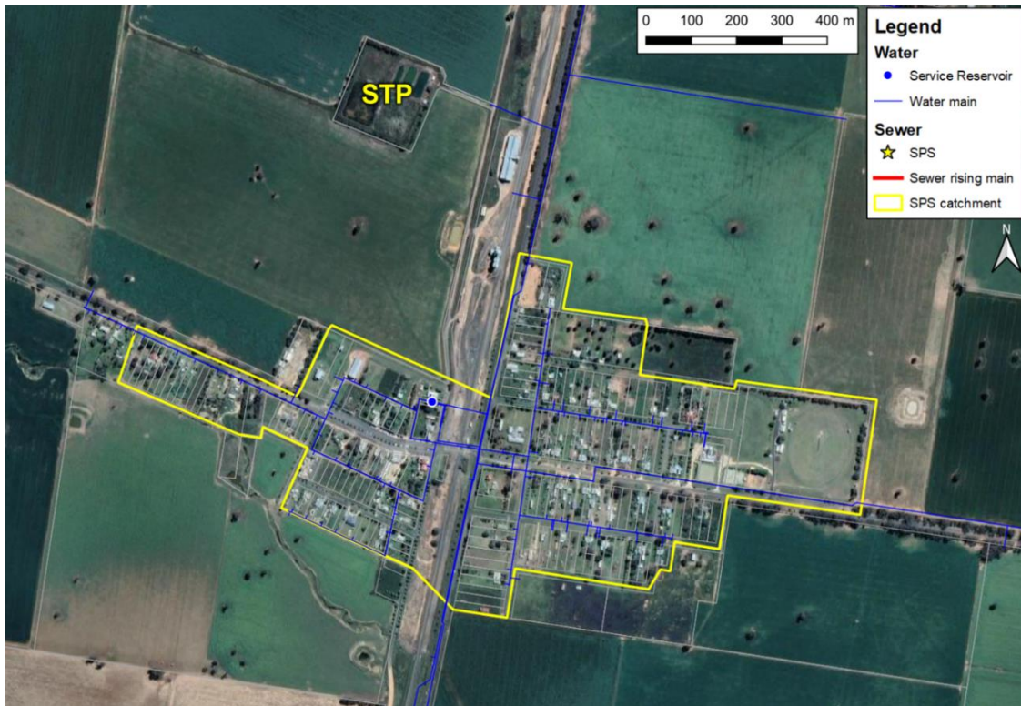
Figure 4-9: Sewerage scheme layout at Yerong Creek with water main overlay
